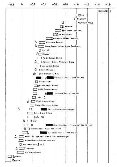
Alloys are listed in the order of the potential they exhibit in flowing seawater. Certain alloys indicated by the symbol in low-velocity or poerly aerated water, and at shielded areas, may become active and exhibit a potential near -0.5 volts.
