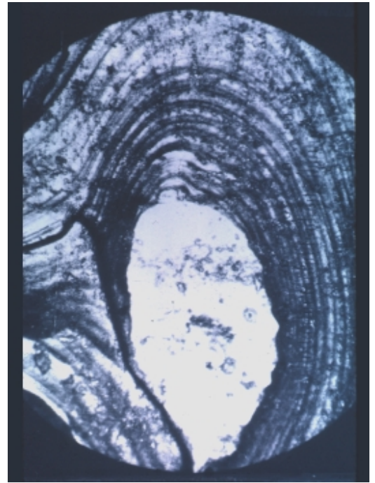
Figure 2 Skip plating defect resembling an oyster shell due to contaminants bleeding from a pore at its bottom. 50X magnification.
