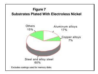
In job shops, most of the work is on ferrous substrates. Approximately 60 percent of the parts that are plated are made from plain steel, iron and alloy steels. This equals a reduction of one quarter from that reported in 1979<sup>18</sup>.
