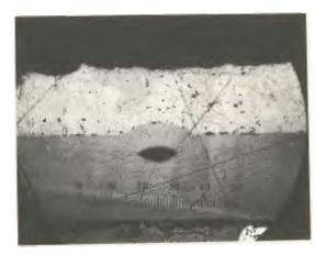
Roughness due to codeposition of particles in the coating.
