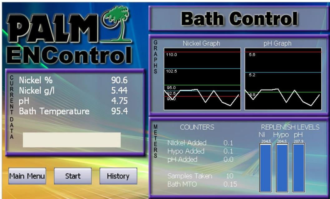
The controller will then flash WAITING FOR START in the status dialog box. The CONTROL screen is divided into three sections.
